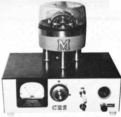
Fig. 2. Sky magnetometer remote sensor (right) and electronics package (above), into which the author has also installed a compass sensor described in Fig. 3.
