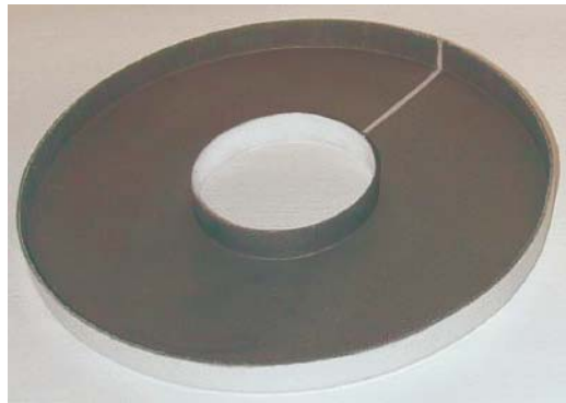
Fig 10: Small gap in the shield
