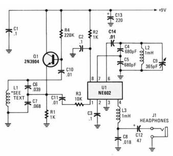
Fig. 2. In this metal-detector circuit, transistor QI (a 2N3904 general-purpose transistor) is configured as a Colpitts oscillator. When sense-loop LI is brought near metal, the loop's inductance changes, shifting the oscillator's operating frequency.
