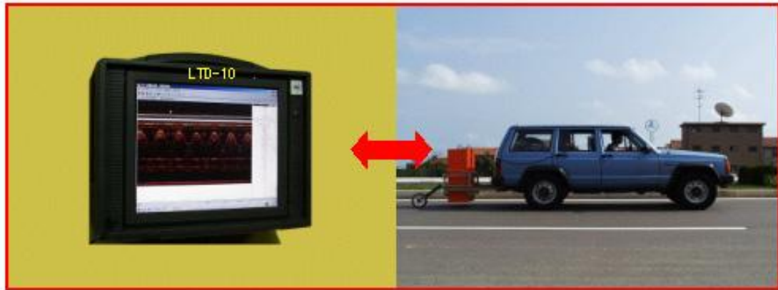
Truck-mounted type of road examination radar system LTD-2000 is at work
